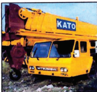
20 TO 30 TONS CRANE
